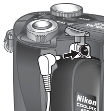
Connecting AC adapter to COOLPIX4500 DC-in connector
